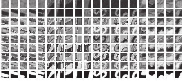
Fig. 4. Feature maps of some patch pairs are produced by the common subnetwork (parameterized by \theta_s ) shared between change detection and reconstruction tasks. The patch pairs are shown in the first and second lines, respectively. From the third line to the eighth line, six (16 in total) feature maps are provided. The predicted CD maps for patch pairs are shown in the last line.
