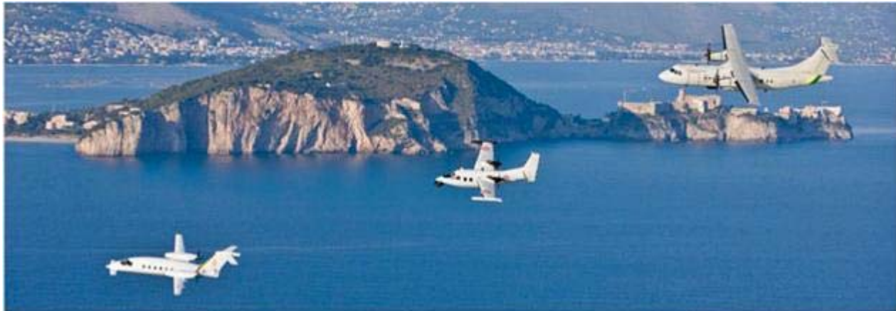
Fig. 2. From the bottom left to the up right: Piaggio P180, Piaggio P166 DP1 and ATR 42MP are the aircrafts available to the Guardia di Finanza Gruppo Esplorazione Aeromarittima based in Pratica di Mare (Rome). They are used every day for maritime patrolling in national and open waters, search and rescue missions, tactical transportation, special operations and airborne remote sensing exploration
