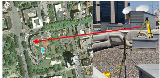
Fig. 6. GPS antenna, materialization of an ' ad hoc ' Station.
