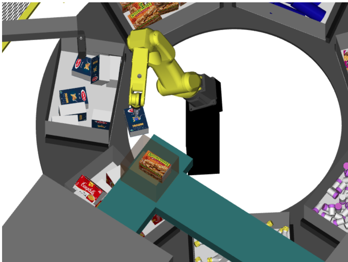
FIGURE 19: Digital twin of robotic work-cell for distributing food
