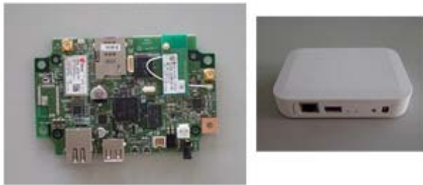
Fig. 3. Digital Grid Controller
