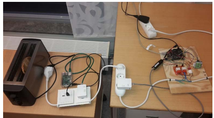
Fig. 5. The prototype implementation. The smart cable to the left connected plugged into the smart socket system to the right.
